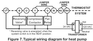
with reversing valve energized in HEAT
